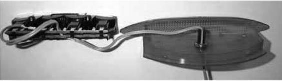
Fig 24 Wire routing through light unit
