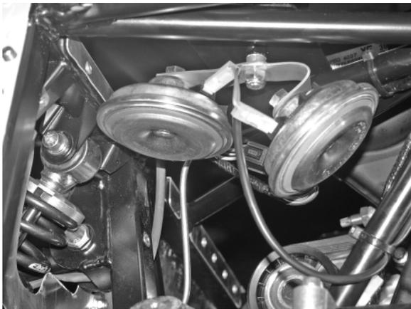
Fig 3 Relocated horns
