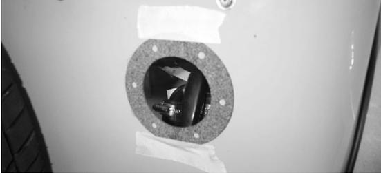
Fig 16 Gasket positioned on back panel
