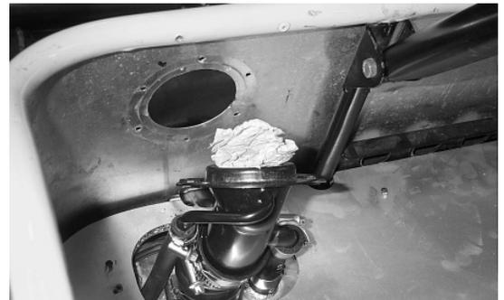
Fig 15 Old filler boss removed
