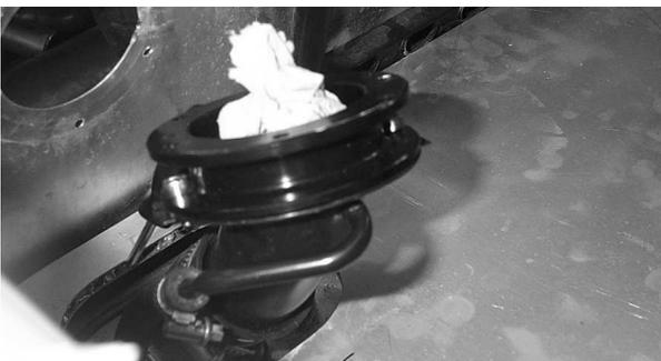
Fig 18 Spacer fitted to filler neck
