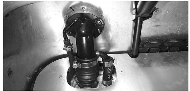
Fig 13 Filler cover and boot carpet removed
