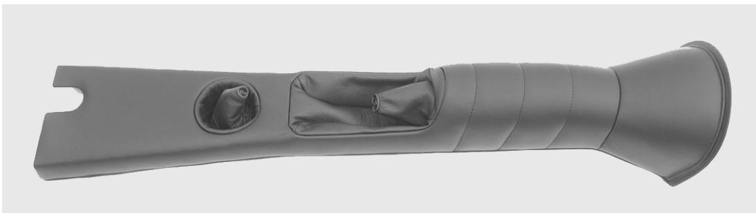
Fig 14 Transmission tunnel top
