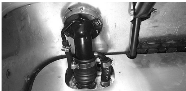
Figure 187: Filler cover and boot carpet removed
