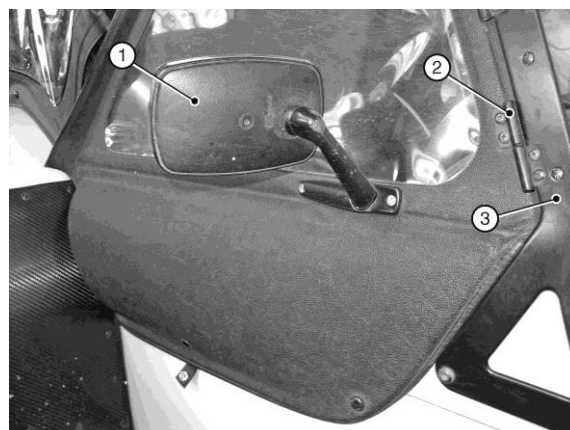
Figure 165: Mirror fitted to side screen
