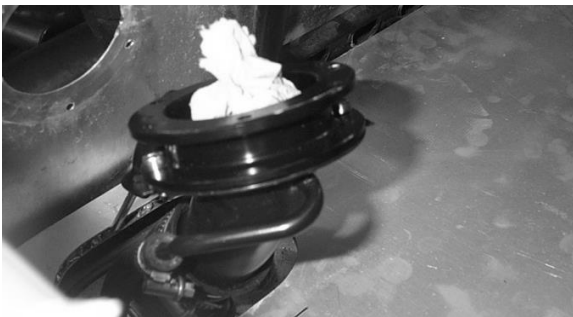
Figure 192: Spacer fitted to filler neck
