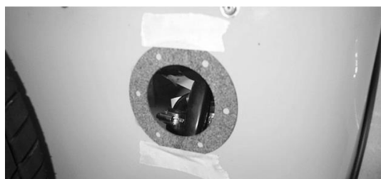
Figure 190: Gasket positioned on back panel
