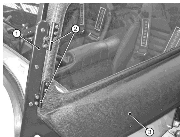
Figure 161: Hinge and side screen fitting
