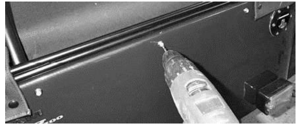
Figure 196: Drilling central popper on SV
