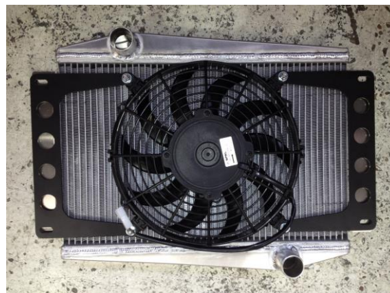
Figure 54: Radiator/fan prior to fitting
