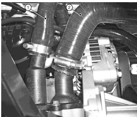
Figure 53: Bottom hose engine connection (viewed from bellow)
