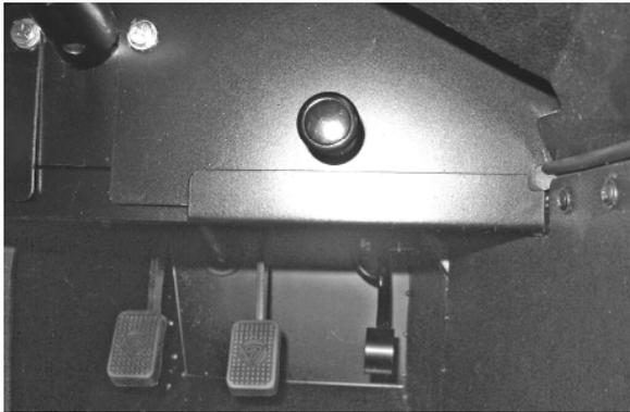
Fig 22 Heater control location
